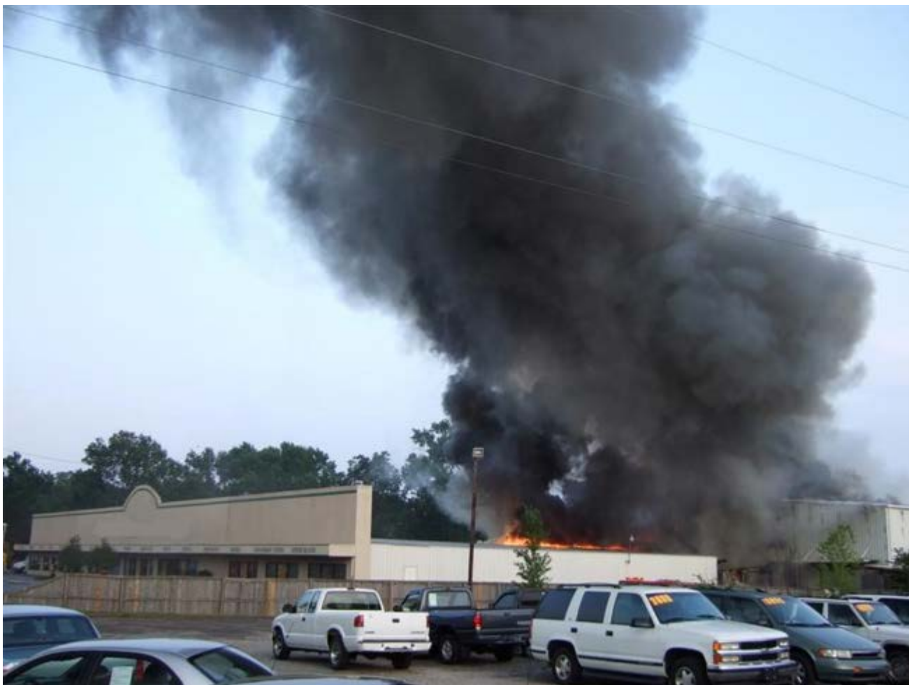
Photo A-1. Time is approximately 1923 hours. Fire is visible over showroom roof. Smoke is dark gray in color and becoming turbulent. The flames may not have been visible from front parking lot or close to the building on the D-side. (Photo courtesy of Dan Folk.)
